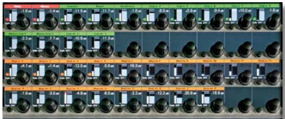
Immediate access of up to 40 master faders with real time meters.
