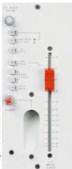
Wedge fader & associated controls
